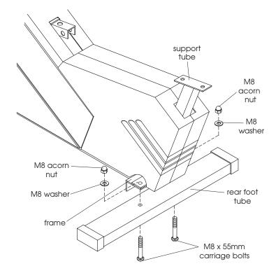
Figure 2 - Install Rear Foot Tube
